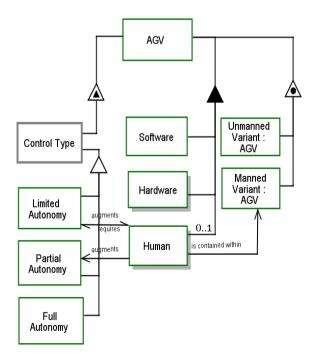
Figure 3: Broad Ground Vehicle Control Type and Manned/Unmanned Classifications
