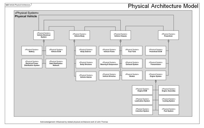
Figure 10: Vehicle Physical Architecture Model
