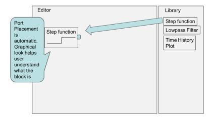
3. **Tailor the library element** – The step function is next tailored. The step is inserted at a time of 1 second and the size of the step is changed to 2 from 1. The Icon adjusts the vertical height of the step to 2. See the diagram below.
